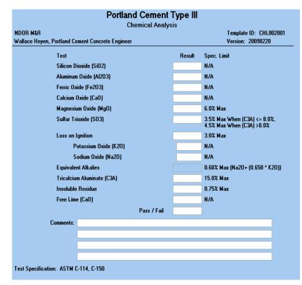
Figure 6, SiteManager Test Template, Portland Cement Concrete, Type III (Chemical Analysis)
