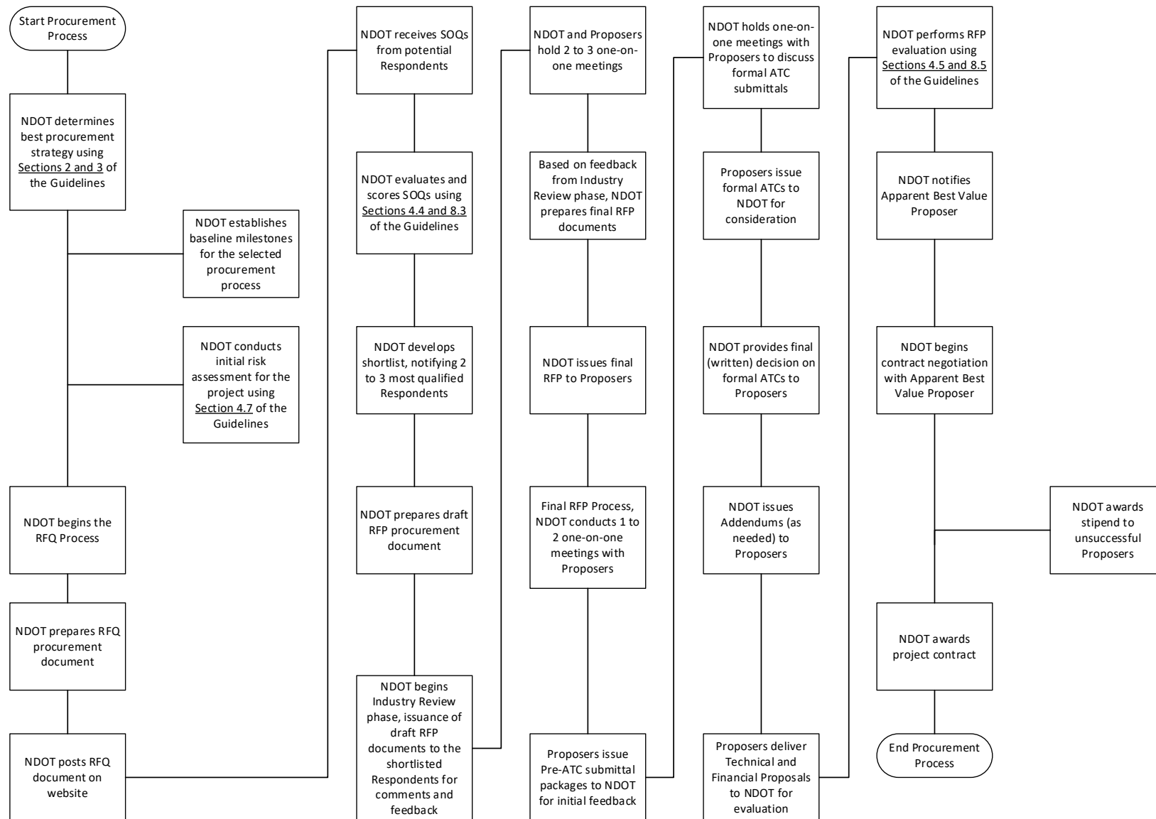
Figure 8-2. P3 Project Delivery Method Procurement Flowchart
