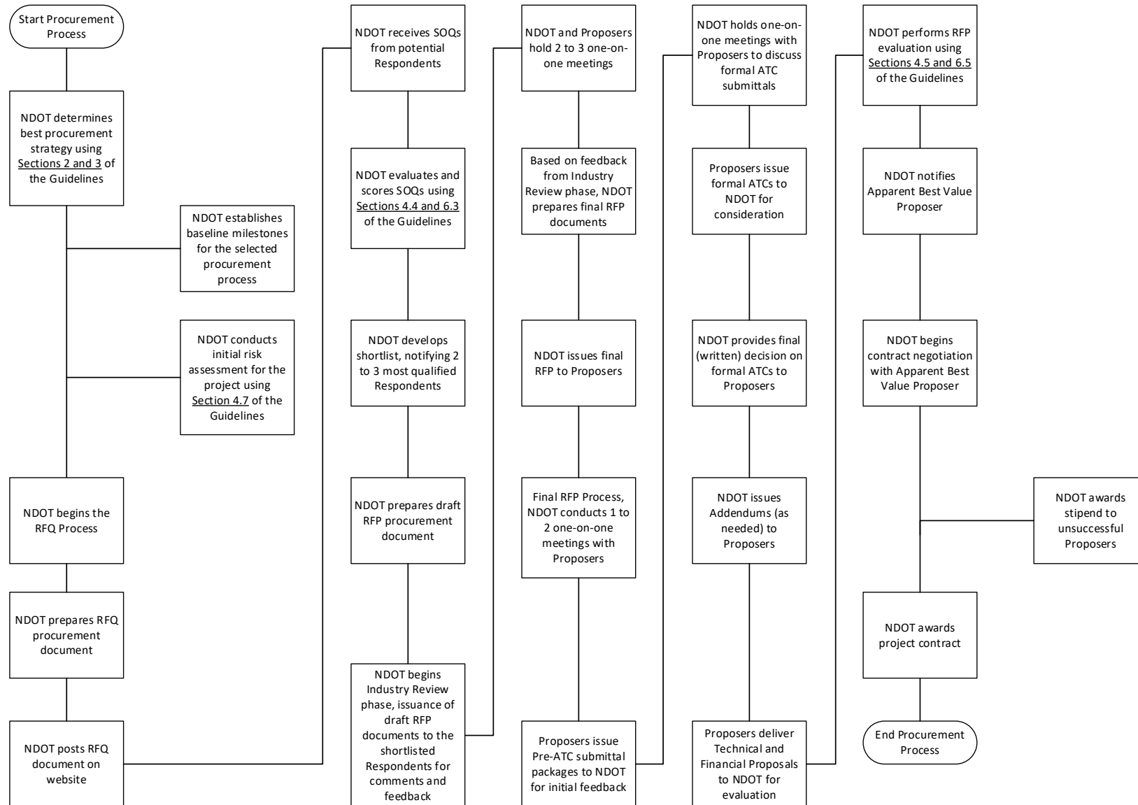
Figure 6-2. DB Project Delivery Method Procurement Process Flowchart
